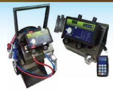
The TT-1 B allows you to do all basic functions remotely with a single mechanic. It is equipped with a wireless remote control with FCC approved technology, with a range of more than 200 feet, without interference or dead zone but does not have an integrated screen. You can therefore activate the electrical and pneumatic circuits remotely. A simple LED is integrated to signal the sending and receipt of the command to the device.
